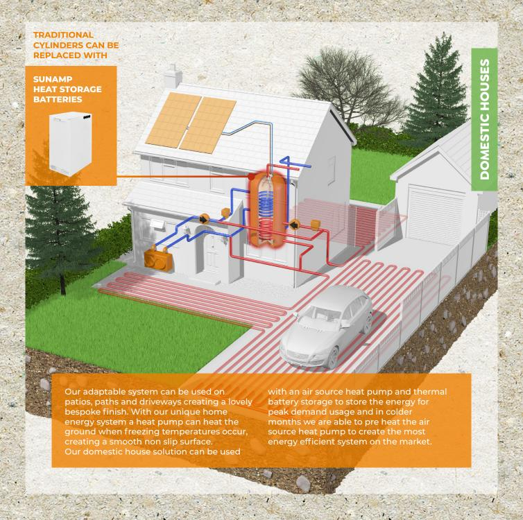
The Addagrip EcoHeat surface is installed onto a suitable base at a depth between 30-45 mm, the Pipework is covered with a larger base stone and the top coat is installed to specific depth and colour choice, it can the be connected to a thermal battery with can store excess heat for peak demand usage
