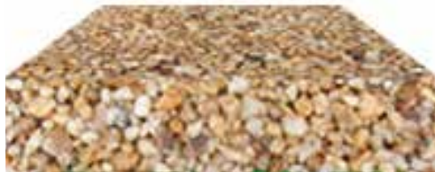
0.5mm dia. grit cast onto uncured surface
